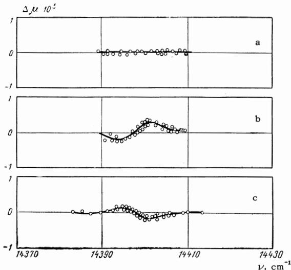
FIG. 4. Dispersion curves: a) without pumping; b) with optical pumping (negative dispersion in ruby  $P_1$ ); c) dispersion curve of ruby  $P_2$  without pumping and with a quartz plate in place of crystal  $P_1$ .
