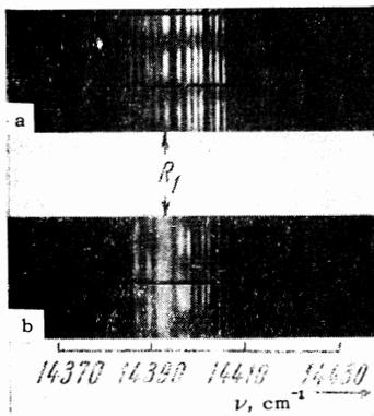
FIG. 3. Interferograms obtained on the set-up described: a) without pumping; b) with optical pumping of crystal  $P_1$ . In the figures each bright vertical band corresponds to a spike of the ruby laser.
