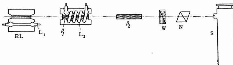
FIG. 1. Optical set-up for observation of dispersion.
