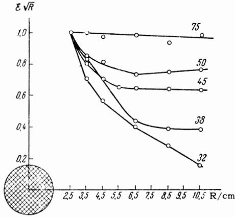
FIG. 8. Dependence of the amplitude of the microwave field  $\mathcal{E}$  on the distance  $R$  to the center of the plasma. The numbers on the curves denote the value of the field  $E_\theta$  in V/cm.
