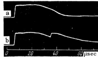
FIG. 3. Blocking of a radio beam of 3 cm wavelength by the plasma: a – following operation of the titanium injectors (shock circuit disconnected), b – following operation of the titanium injectors and the shock circuit.
