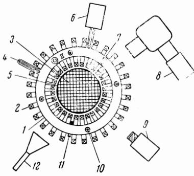
FIG. 1. Diagram of setup: 1 – glass chamber, 2 – coils of quasistationary magnetic field, 3 – high-frequency shock circuit, 4 – probe for measuring transverse velocities of the electrons and ions, 5 – carbon cylinder, 6 – x-ray pickup, 7 – microwave sounding of the plasma at 3 cm wavelength, 8 – monochromator, 9 – hard gamma radiation pickup, 10 – titanium injectors, 11 – Rogowski loop, 12 – horn for the investigation of microwave radiation of the plasma.
