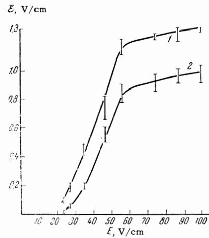
FIG. 7. Dependence of the amplitude of the microwave field on the electric field  $E_\theta$ .
