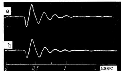
FIG. 4. Oscillograms of electric field  $E_\theta$  (a) and of the current (b).
