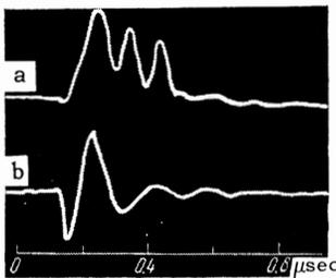
FIG. 6. Oscillograms of microwave signal from a plasma (a) and oscillograms of the current (b).
