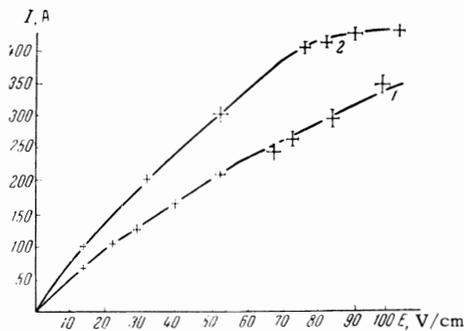
FIG. 5. Dependence of the discharge current on the loop voltage.
