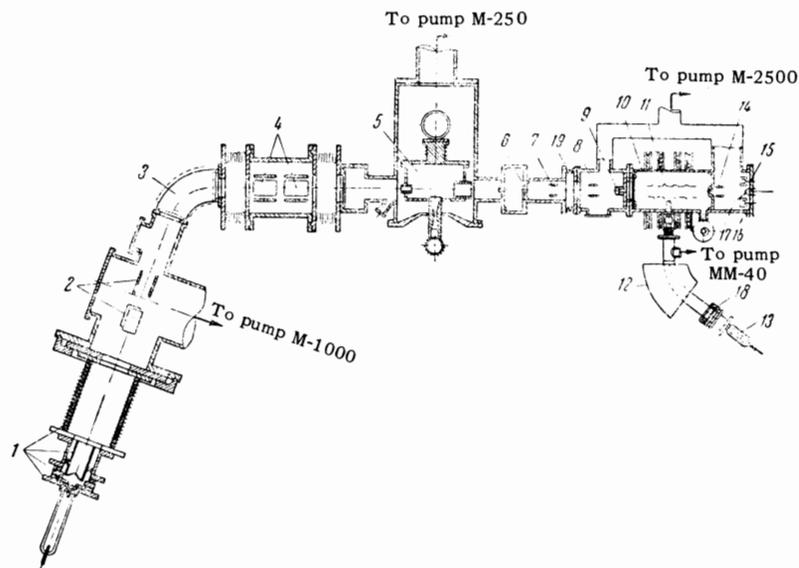
the gas filling the collision chamber by a transverse electric field was accomplished by a mass spectrometer 12 connected to the side of the chamber.
