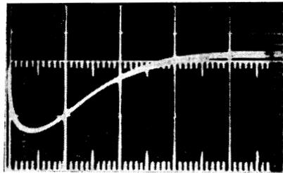
FIG. 2. Shape of the magnetic field pulse (time scale—100  $\mu$ sec per large division).
