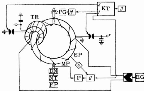
FIG. 1. Schematic diagram of the apparatus: TR, toroidal transformer; PG, M, pre-ionization generator and modulator; DN, NT, FP, pumping system; MP, magnetic probe; KT, Z, synchronization unit; EP, double electric probe; EG, excitation generator; P, O, preamplifier and oscilloscope.
