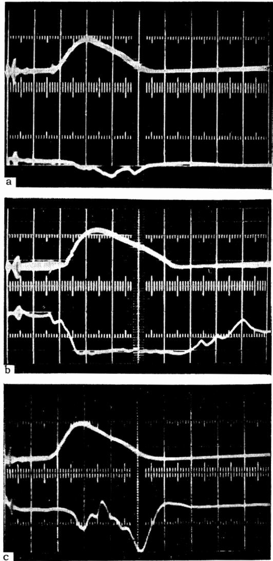
FIG. 4. Oscillograms of the current in the chamber and the signal from the magnetic probe: a—no excitation, magnetic field and current on; b—excitation applied, no magnetic field; c—magnetic field, hf excitation, and current all on.
