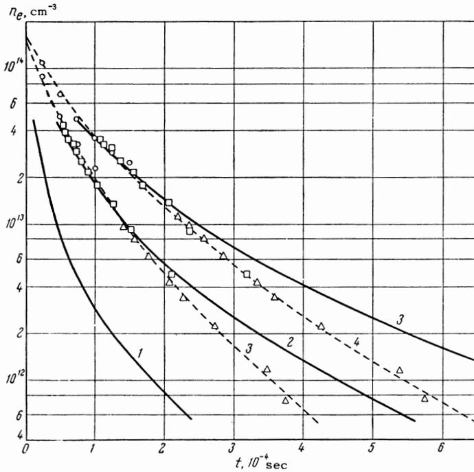
FIG. 2. Decay curves of electron density in a plasma:  $\circ$  – data of the Fabry-Perot interferometer;  $\square$  – data of the microwave interferometer for  $\lambda = 4$  mm;  $\triangle$  – data of the microwave interferometer for  $\lambda = 8$  mm. The curve 1 –  $H = 100$  Oe, 2 –  $H = 300$  Oe, 3 –  $H = 500$  Oe, 4 –  $H = 1200$  Oe. (dashed curves – helium with hydrogen in the ratio 6:4, solid curves – helium).
