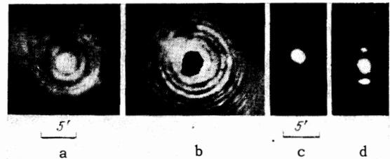
FIG. 3. Far field pattern of the emission from a well-aligned sample. a – normal exposure; b – increased ring contrast obtained by screening out the central spot; c – for the case where the total radiation is strongly attenuated; d – for the case where the sample is inclined by  $1'$  to the axis of the cavity.
