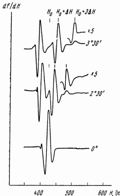
FIG. 1. Size-effect line vs. the inclination of the field,  $n \parallel [010]$ , accurate to  $1^\circ$ ,  $d = 0.40 \text{ mm}$ . The high-frequency electric-field vector is  $E \parallel [100]$ , the angle between  $[001]$  and the projection of  $H$  on the plane of the sample is  $3^\circ$ . Weak lines are plotted in addition with a magnification of 5x.
