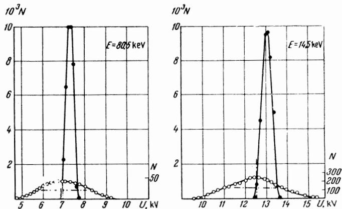
FIG. 2. Distribution of particles in a beam as a function of the voltage across the electrostatic analyzer: ● — in the absence of a film; ○ — after passing through a film.
