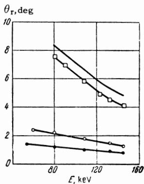
FIG. 5. Dependence of the angle of the resultant deviation on the energy of  $\text{Li}^+$  ions: ● — in a celluloid film  $2 \mu\text{g}/\text{cm}^2$  thick; ○ — in a celluloid film  $6 \mu\text{g}/\text{cm}^2$  thick; □ — in a carbon film  $17 \mu\text{g}/\text{cm}^2$  thick; continuous curve represents the data from [6].
