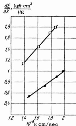
FIG. 6. Dependence of the specific energy loss on the velocity of  $\text{Li}^+$  ions: ● — in a celluloid target; □ — in a carbon target.
