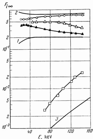
FIG. 3. Dependence of the equilibrium charged fractions on the energy of  $Li^+$  ions;  $\Delta$ ,  $\circ$ ,  $\square$  -  $F_{0\infty}$ ,  $F_{1\infty}$ ,  $F_{2\infty}$ , respectively, for a celluloid film;  $\triangle$  -  $F_{0\infty}$  for a carbon film. Curves 1, 2, and 3 represent  $F_{0\infty}$ ,  $F_{1\infty}$  and  $F_{2\infty}$  for gaseous nitrogen, taken from<sup>[1]</sup>.
