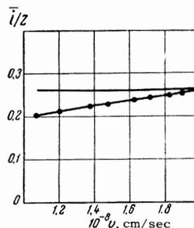
FIG. 4. Dependence of the degree of ionization on the velocity of  $Li^+$  ions:  $\bullet$  - for a celluloid film; continuous curve - for gaseous nitrogen, taken from<sup>[1]</sup>.
