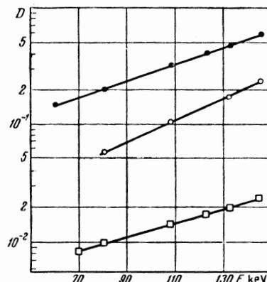
FIG. 7. Dependence of the transmission of the beam on the energy of the  $\text{Li}^+$  ions: ●, ○ — for celluloid films 2 and 6  $\mu\text{g}/\text{cm}^2$  thick, respectively; □ — for a carbon film  $17 \mu\text{g}/\text{cm}^2$  thick.
