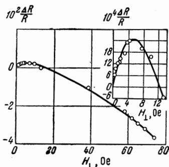
FIG. 5. Relative change of the electrical resistance of iron in weak transverse fields;  $T = 4.2^\circ\text{K}$ .
