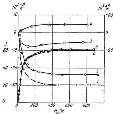
FIG. 1. The dependence, on an external longitudinal field, of the relative electrical resistance  $\Delta R/R$  of iron at temperatures of 4.2°K (1), 20.4°K (2), 77°K (3) and 293°K (4), and of the magnetization of iron  $J$  (in arbitrary units) at 4.2°K (5) and 293°K (6). The scale on the right applies to curves 3 and 4.
