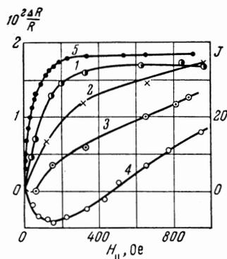
FIG. 3. Dependence, on an external longitudinal magnetic field, of the relative electrical resistance  $\Delta R/R$  of nickel at  $4.2^\circ\text{K}$  (1),  $20.4^\circ\text{K}$  (2),  $77^\circ\text{K}$  (3),  $293^\circ\text{K}$  (4), and of the magnetization  $J$  at  $4.2^\circ\text{K}$  (5) and  $293^\circ\text{K}$  (6).
