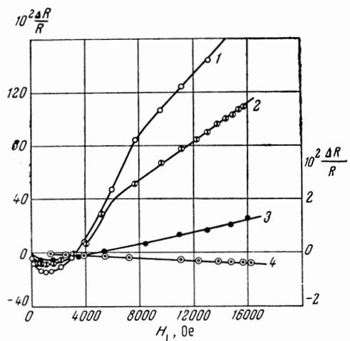
FIG. 4. Relative change of the electrical resistance of iron in a transverse magnetic field at  $4.2^\circ\text{K}$  (1),  $20.4^\circ\text{K}$  (2),  $77^\circ\text{K}$  (3),  $293^\circ\text{K}$  (4); the scale on the right applies to curves 3 and 4.
