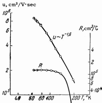
FIG. 4. Temperature dependence of the electron mobility and of the Hall coefficient for sample No. 1.
