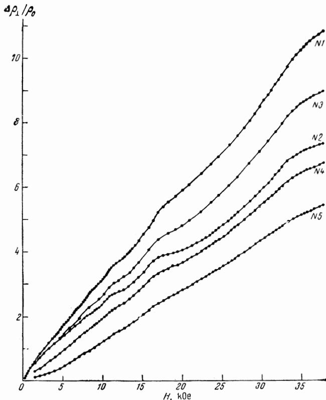
FIG. 5. Transverse magnetoresistance curves obtained at  $T = 90^\circ\text{K}$ , for n-InSb samples with different carrier densities. The curves demonstrate the independence of the period and of the phase of the modulation of the concentration.
