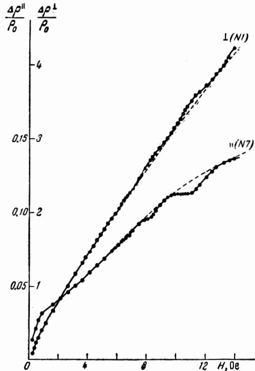
FIG. 2. Curves of transverse and longitudinal magnetoresistance, obtained in the investigation of samples n-InSb No. 1 and No. 7 at  $T = 90^\circ\text{K}$ .
