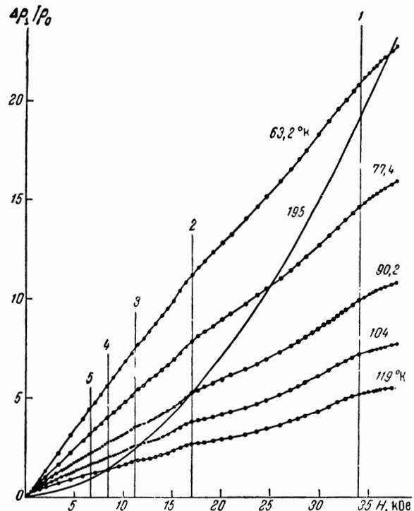
FIG. 3. Curves of transverse magnetoresistance, obtained in the investigation of sample No. 1 of n-InSb at different temperatures. The vertical lines with integer indices  $M = 1 - 5$  indicate the magnetic field intensity values corresponding to the resonant condition  $\omega = MeH/m^*c$ .
