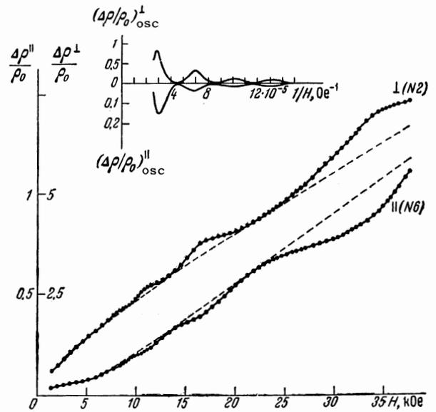
FIG. 1. Curves showing the transverse ( $\Delta\rho_{\perp}/\rho_0$ ) and longitudinal ( $\Delta\rho_{\parallel}/\rho_0$ ) magnetoresistance, obtained in the investigation of samples of n-InSb (No. 2 and No. 6) at  $T = 90^\circ\text{K}$ . The dashed lines represent the monotonic background, on which the resonant oscillations are superimposed. In the upper part of the figure is shown the oscillating part of the magnetoresistance as a function of the reciprocal field intensity.
