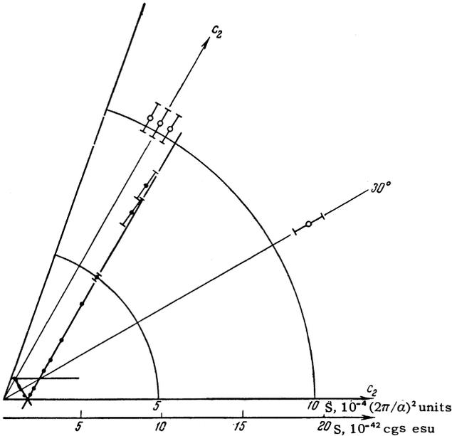
FIG. 3. Anisotropy of the extremal cross sections of the Fermi surface of bismuth in the  $(c_1, c_2)$  plane:  $\circ$  – holes,  $\bullet$  – electrons. The errors of measurements are shown for the large cross sections. For the remaining points, the error is represented by the dimension of the point.
