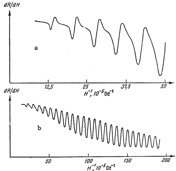
FIG. 4. Change of the form of the oscillations on increase of the magnetic field intensity. Both curves have been recorded for the same direction of the magnetic field ( $H \parallel c_2$ ). In recording the upper curve, the scale has been extended along the axis of the reciprocal of the magnetic field and the amplification has been increased.
