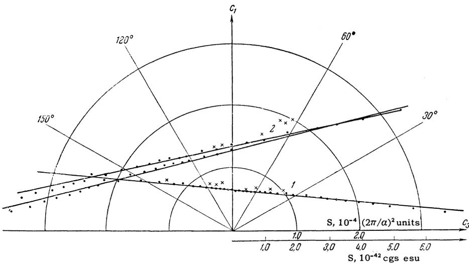
FIG. 2. Anisotropy of the extremal cross sections of the electron Fermi surface of bismuth obtained for the  $(c_1, c_3)$  plane; it shows part of Fig. 1 on a larger scale. Crosses represent the results of Brandt et al.<sup>[5]</sup>
