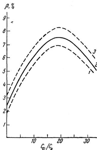
Dependence of the correlation coefficient on  $C_P/C_A$ , calculated for the following values of  $\Delta$ : 1 - 0, 2 - 1.9, and 3 - 3.
