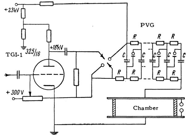
FIG. 1. Circuit for pulse supply of the chamber
