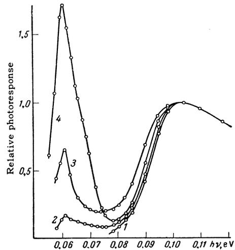
Photoconductivity spectrum of Ge:Zn:Sb. Zinc concentration (in  $\text{cm}^{-3}$ ): 1)  $1.2 \times 10^{15}$ ; 2)  $1.6 \times 10^{16}$ ; 3)  $4 \times 10^{16}$ ; 4)  $3 \times 10^{17}$ . Field 50 V/cm,  $T = 4.2^\circ\text{K}$ .
