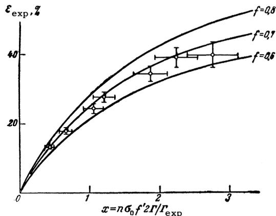
FIG. 1. Dependence of Mössbauer effect  $\epsilon_{\text{exp}}$  at room temperature on absorber thickness  $x$ . The source of the radiation is  $\text{Fe}^{57\text{m}}$  in a gold lattice, the absorber is stainless steel.
