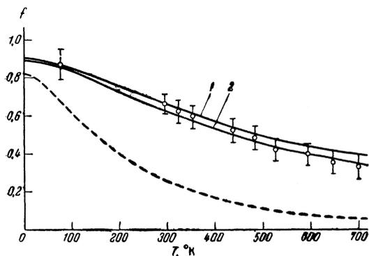
FIG. 2. Temperature dependence of probability  $f$  for resonance emission of 14.4 keV  $\gamma$  quanta by impurity  $\text{Fe}^{57\text{m}}$  nuclei in a gold lattice.
