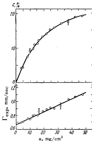
FIG. 3. Dependence of resonance absorption effect  $\epsilon$  and observed line width  $\Gamma_{exp}$  on absorber thickness  $a$  for an  $Mg_2Sn$  absorber at room temperature. The curves were calculated theoretically using the parameter values given in the text.
