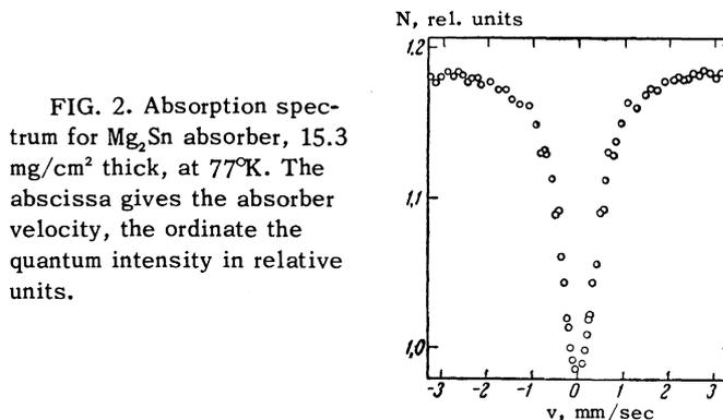
FIG. 2. Absorption spectrum for  $Mg_2Sn$  absorber,  $15.3 \text{ mg/cm}^2$  thick, at 77°K. The abscissa gives the absorber velocity, the ordinate the quantum intensity in relative units.
