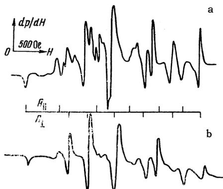
Spectra of isotropic hfs EPR lines from  $\text{Re}^{185}$  and  $\text{Re}^{187}$  in low-temperature glasses containing 0.1 mole per liter of  $\text{ReOCl}_4$  ( $\nu = 9320$  Mc,  $T = 77^\circ\text{K}$ ): a—sulfuric-acid glass, b—dioxane.
