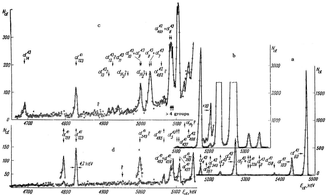
FIG. 1. Spectrograms of  $\alpha$  radiation from  $\text{Am}^{241-243}$ . The ordinates represent the number of  $\alpha$ -particle tracks per 1-mm length of the photographic plate.
