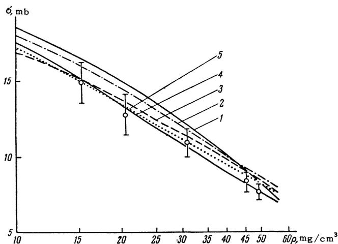
FIG. 3. Calculated resonant scattering cross section vs. density: 1— $\tau_2 = 7.1 \times 10^{-12} \text{ sec}$ , 2— $\tau_2 = 3.55 \times 10^{-12} \text{ sec}$ , 3— $\tau_2 = 2.37 \times 10^{-12} \text{ sec}$ , 4— $\tau_2 = 1.78 \times 10^{-12} \text{ sec}$ , 5— $\tau_2 = 0$ . Points—experimental data.
