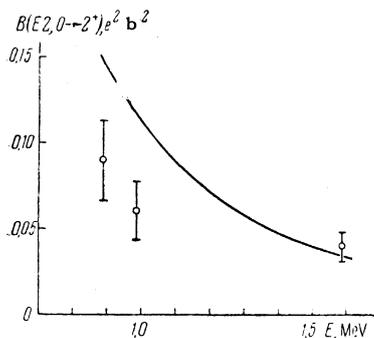
FIG. 4. Energy dependence of  $B(E2, 0 \rightarrow 2^+)$  for the isotopes of Ti ( $\text{Ti}^{46}$ <sup>[8]</sup>,  $\text{Ti}^{48}$ <sup>[9]</sup>,  $\text{Ti}^{50}$ <sup>[22]</sup>). Solid curve — calculation by the pair-correlation model,<sup>[17]</sup> points — experimental data.
