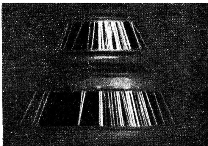
FIG. 1. Electron shower recorded in the spark chambers.
