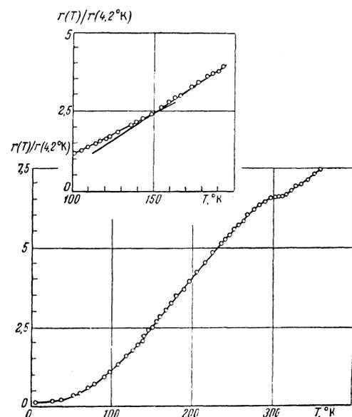
FIG. 1. Temperature dependence of electric resistivity of a chromium sample with ratio  $\rho = 6.4$ .
