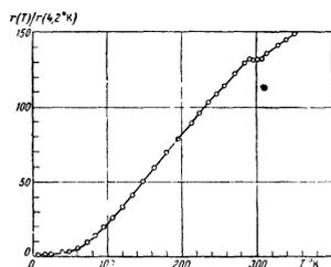
FIG. 2. Temperature dependence of electric resistivity of a chromium sample with ratio  $\rho = 130$ .
