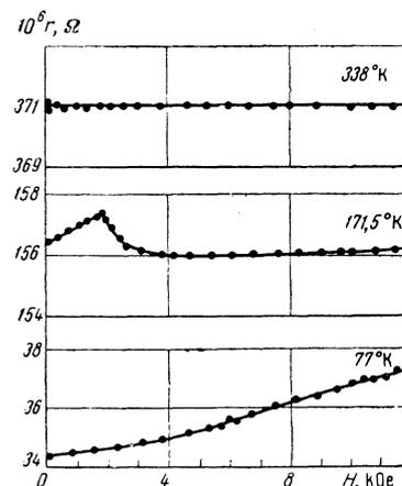
FIG. 4. Dependence of electric resistivity on the external magnetic field  $H$  for a chromium sample with  $\rho = 130$  at different temperatures.
