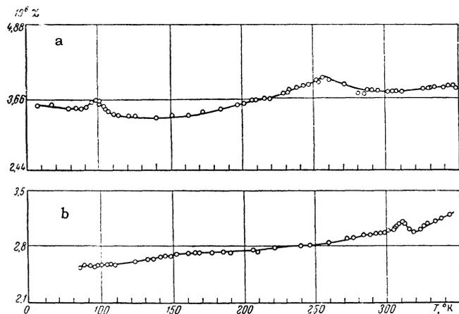
FIG. 3. Temperature dependence of the magnetic susceptibility of chromium samples with  $\rho = 6.4$  (a) and 130 (b).
