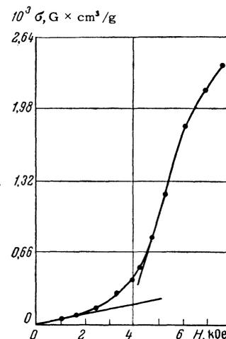
FIG. 5. Dependence of magnetization on the field for a sample with  $\rho = 130$  at 196°K.
