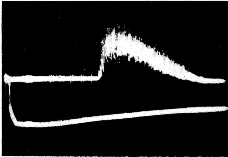
FIG. 1. An oscillogram of the output of the crystal (top trace). The modulation, which decreases during the pulse, is clearly visible. The bottom trace shows the pulse of the flash lamp.
