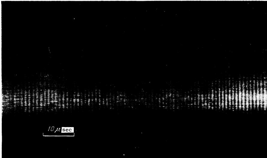
FIG. 2. Time sweep of the output of the ruby laser. Each bright band is a spike.
