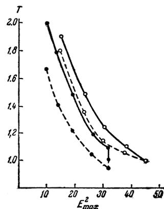
FIG. 3. The dependence of the period  $T$  on  $E_{max}^2$  for two different crystals with the laser operated at low temperature ( $108^\circ K$ ) and close to threshold. (The voltage on the flash lamp was 2.6 kV, the threshold voltage 2.5 kV.) The experimental dependence is shown by the solid lines, and the theoretical dependence by the dashed lines (the units are arbitrary).
