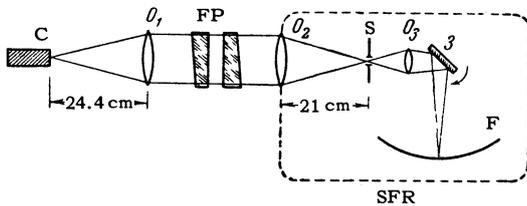
FIG. 4. Arrangement for time-scanning the emission spectra.
