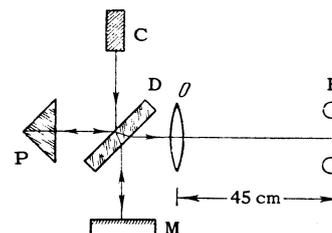
Similarly, one can study the coherence of the radiation from different parts of the end surface. For this, it is necessary to place between the crystal  $C$  and the beam divider  $D$  (Fig. 1) another objective at its focal distance from the end of  $C$ . In this case, one obtains two superposed images of the end in the plane  $F$ . This method makes it possible to investigate the coherence over the whole field at once.
