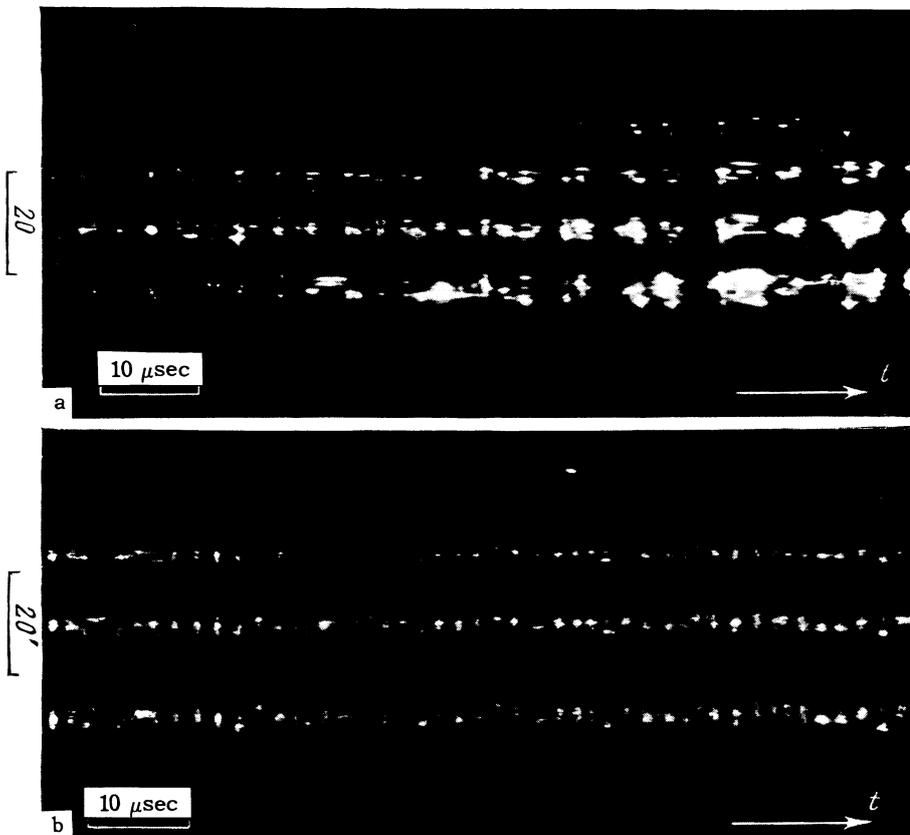
FIG. 5. Scan of the spectra of radiation being propagated in different directions. The same ruby as in Fig. 3. Separation between Fabry-Perot plates, 5 mm. a – temperature of the ruby,  $20^\circ\text{C}$ . Initiation of generation. b – temperature of the ruby,  $-165^\circ\text{C}$ . Thirty microseconds after initiation.
