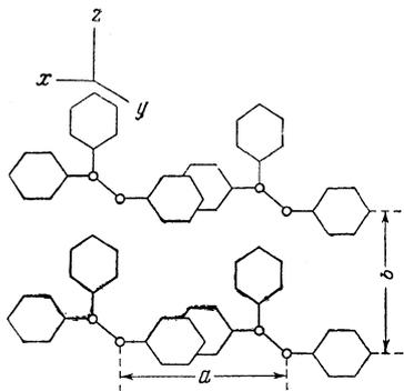
Model of the crystal lattice of the free radical  $\alpha\alpha$ -diphenyl- $\beta$ -picrylhydrazyl. The lattice consists of layers of this kind, somewhat displaced relative to each other, O-N atoms.
