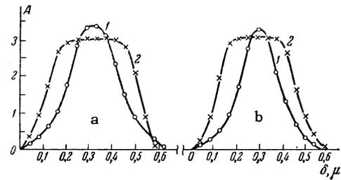
FIG. 9. Effect of tension on a domain wall in silicon iron. The load was applied: a) along the wall; b) at right angles to the wall. Curves 1 represent walls in unloaded state, curves 2 under a load.
