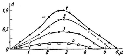
FIG. 10. Effect of compression on a 180° wall in nickel. The direction of the compression is along the wall. Curve 1 - zero load; 2)  $\sigma = 0.5 \text{ kg/mm}^2$ ; 3)  $\sigma = 2 \text{ kg/mm}^2$ ; 4)  $\sigma = 4 \text{ kg/mm}^2$ .
