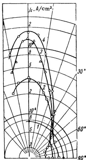
FIG. 1. The dependence of critical current density  $j_c$  on the angle between the plane of rolling and the external field ( $H = 23.5$  kOe,  $T = 4.2^\circ\text{K}$ , alloy Nb + Zr (25%)): 1 - recrystallized specimen, 2 - deformation 80%, 3 - 95.5%, 4 - 97.8%.
