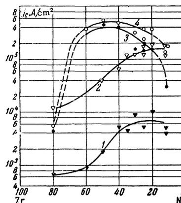
FIG. 3. The values of  $j_{c\parallel}$  and  $j_{c\perp}$  in a field of 23.5 kOe for cold-deformed specimens and specimens annealed at  $600\text{--}800^\circ\text{C}$  with various compositions ( $T = 4.2^\circ\text{K}$ ): 1 -  $j_{c\perp}$ , 2 -  $j_{c\parallel}$  (cold-deformed specimens), 3 -  $j_{c\perp}$ , 4 -  $j_{c\parallel}$  (annealed specimens).
