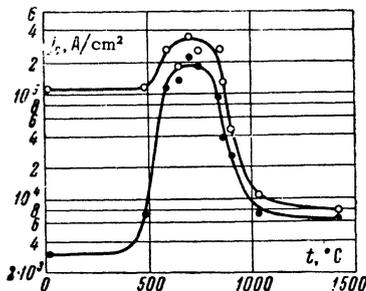
FIG. 4. The variation of  $j_{c||}$  and  $j_{c\perp}$  in a field of 23.5 kOe with annealing temperature  $t$  (alloy Nb + Zr (25%),  $T = 4.2^\circ\text{K}$ ).
