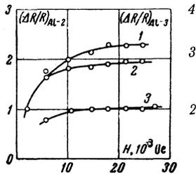
FIG. 3. Dependence of the change in the resistance on the magnetic field: 1)  $\Delta R/R$  for Al-2,  $\varphi = 20^\circ$ ; 2)  $\Delta R/R$  for Al-2,  $\varphi = 60^\circ$ ; 3)  $\Delta R$  for Al-3.
