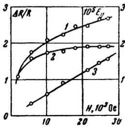
FIG. 2. Dependence of the change in the resistance and Hall field on the magnetic field for sample Al-1: 1)  $\Delta R/R$ ,  $\varphi = 130^\circ$  (max.); 2)  $\Delta R/R$ ,  $\varphi = 40^\circ$  (min.); 3)  $E_y$ .
