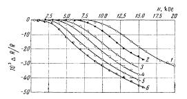
FIG. 4. Dependence of  $\Delta R/R$  on H. Curve 1 – atmospheric pressure; curves 2-6 at pressures (P) 2600, 5400, 7025, 8850, and 10800 kg/cm<sup>2</sup>, respectively.
