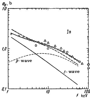
FIG. 2. Comparison of the experimental cross sections for neutron capture in In with the theoretical curves. The solid curve is calculated from the results of the second in the series of calculations (see the table), while the dashed curve is from the results of the first series. We also give the partial capture cross sections due to s- and p-neutrons (second series of calculations):  $\circ$  – experimental points from [13],  $\square$  – from [5], and  $\Delta$  – from [6].
