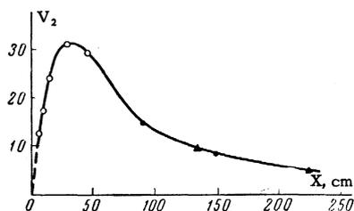
FIG. 1. Dependence of the pressure amplitude (the voltage  $V_2$  on the receiver plate, in mV) of the second harmonic (10 Mc) on the distance from the radiator in the alloy MA-8 with 1000 V (peak) across the radiator: ○ – from the amplitude of the first pulse for rods of various lengths; ● – from the second and third pulses for a rod of 30 cm length; ▲ – from the second and third pulses for a rod of 45 cm length.
