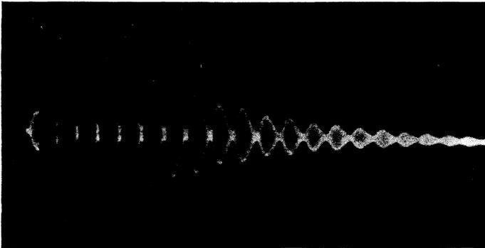
FIG. 3. Series of pulses exponentially decaying in amplitude for the same sample as in Fig. 2 but when 30 V were applied to a radiator plate with a natural frequency of 10 Mc; the signal was received using a plate with the same natural frequency 10 Mc.
