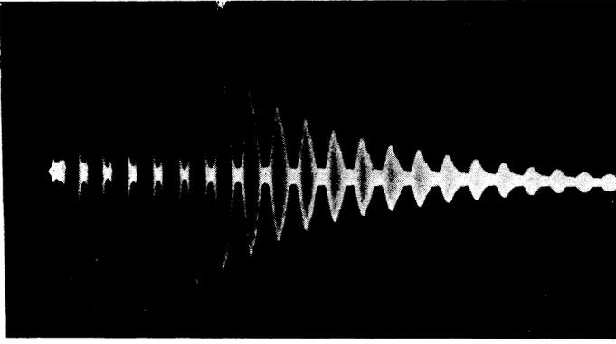
FIG. 2. Series of second-harmonic (10 Mc) pulses arising and then decaying in amplitude in an MA-8 rod of 7.5 cm length. The voltage across the radiator (5 Mc) was 1000 V (peak).
