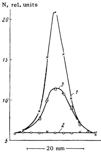
FIG. 1. Dependence on source temperature for the integral counting rate from two different sections of the source: 1, 2 – cold source, 3 – hot source ( $\square, \times$ , first section;  $\circ, \Delta$ , second section).
