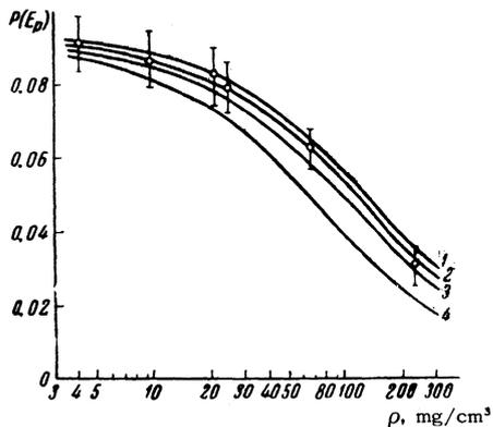
FIG. 3. Dependence of  $P(E_p)$  (number of quanta per eV near  $E = E_p$ ) on source density. Curves computed from formula (1): 1 -  $\tau_2 = 1 \times 10^{-12}$  sec; 2 -  $\tau_2 = 7.5 \times 10^{-12}$  sec; 3 -  $\tau_2 = 15 \times 10^{-12}$  sec; 4 -  $\tau_2 = 45 \times 10^{-12}$  sec. The circles are the experimental data.
