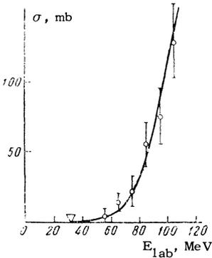
FIG. 4. Cross section for the reaction  $C^{12} + C^{12} \rightarrow 6\alpha$  as a function of carbon ion energy in the laboratory system.
