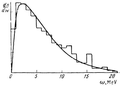
FIG. 3. Energy distribution of  $\alpha$  particles from the reaction  $C^{12} + C^{12} \rightarrow 6\alpha$ .
