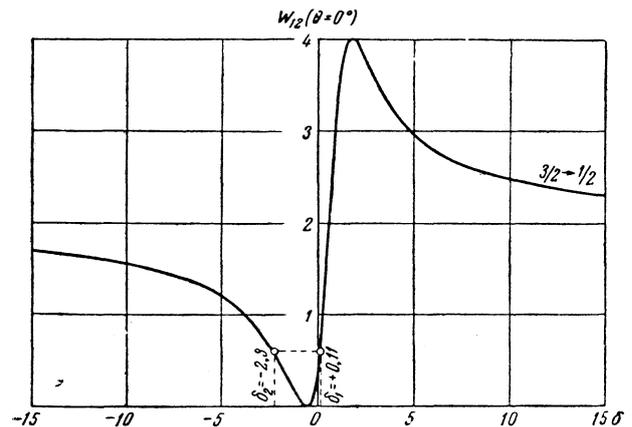
FIG. 1. Dependence of the gamma-ray intensity on the mixture coefficient  $\delta$  for the  $3/2 \rightarrow 1/2$  transition ( $\theta = 0$ , M1 + E2 mixture). Both values of  $\delta$  correspond to an angular distribution  $1 - 0.40 \cos^2 \theta$ <sup>[6]</sup> of the gamma rays from the reaction  $Si^{30}(p, \gamma)P^{31}$  for the transition of the resonant 8.04-MeV level to the ground level of the  $P^{31}$  nucleus ( $E_p = 773 \text{ keV}$ ).
