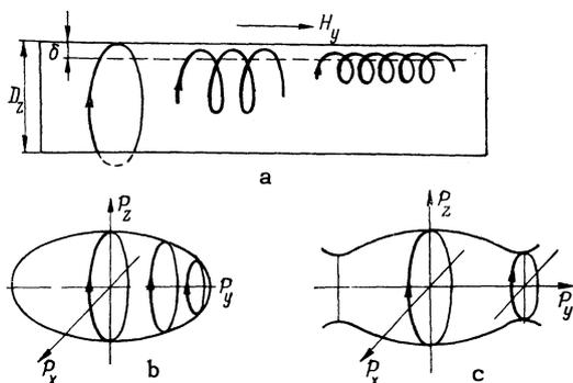
FIG. 3. Illustration of the phenomenon of cutting-off non-resonance electron orbits by the surface of a thin specimen.
