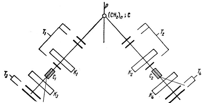
FIG. 1. Schematic diagram of the experiment for measurement of  $C_{kp}$ :  $C_1$  and  $C_2$  - analyzing target;  $K_1, K_2, K_3, K_4$  - gas discharge chambers;  $T_1, T_2, T_3, T_4$  - scintillation counter telescopes.
