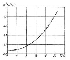
FIG. 3. Temperature dependence of the electrical resistance of iron with the earth's field compensated.
