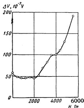
FIG. 6. The dependence of the photo-response  $\Delta V$  on the magnetic field applied along the specimen axis.
