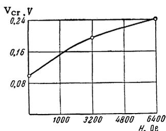
FIG. 7. The dependence of the signal break voltage on the applied magnetic field (the curve corresponds to the end points of the curves in Fig. 4).
