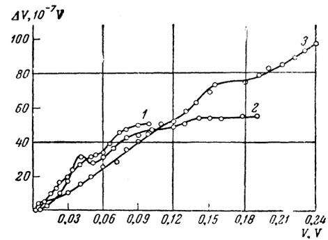
FIG. 4. The variation of photo-response  $\Delta V$  with the voltage applied to the specimen for various magnetic fields: 1— $H = 0$ ; 2— $H = 3200$ ; 3— $H = 5100$  Oe.
