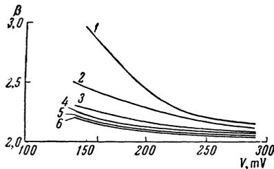
FIG. 3. The variation of  $\beta$  with applied voltage for various values of magnetic field: 1— $H = 0$ ; 2— $H = 1000$ ; 3— $H = 2000$ ; 4— $H = 3000$ ; 5— $H = 4000$ ; 6— $H = 5400$  Oe.
