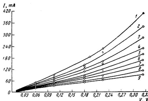
FIG. 2. Voltage-current characteristics for various strengths of applied magnetic field: 1 - H = 0; 2 - H = 800; 3 - H = 1600; 4 - H = 2400; 5 - H = 3200; 6 - H = 4000; 7 - H = 4800; 8 - H = 5600; 9 - H = 6400 Oe.
