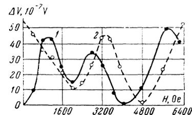
FIG. 5. The dependence of photo-response  $\Delta V$  on the applied transverse magnetic field: 1— with zero external electric field; 2— with an external electric field.
