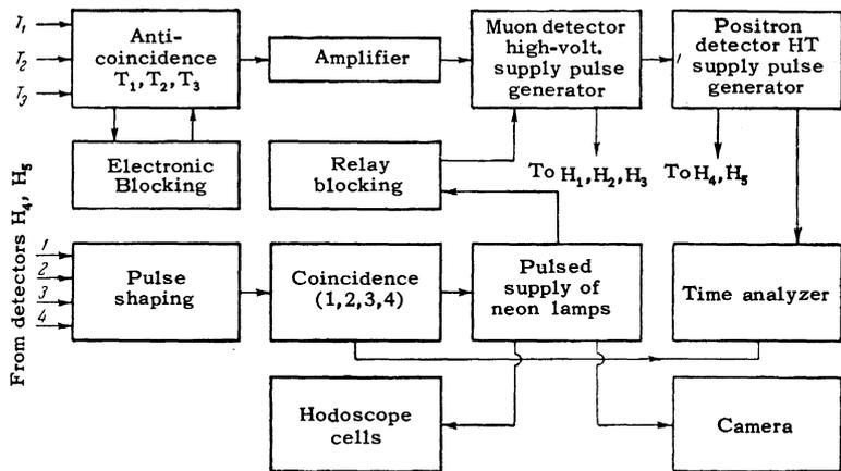
FIG. 2. Block diagram of the electronic circuitry.
