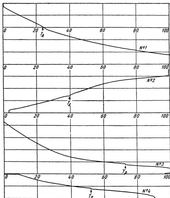
FIG. 2. Typical heating (1) and cooling (2) curves as recorded by the EPP-09 potentiometer. The breaks correspond to  $T_\lambda$ . Curve 1 refers to a mixture having a  $\text{He}^3$  concentration of 59.6%, curve 2, to a 50.0% mixture. Phase separation of the mixtures is recorded on curves 3 (66.1%  $\text{He}^3$ ) and 4 (62.4%  $\text{He}^3$ ).
