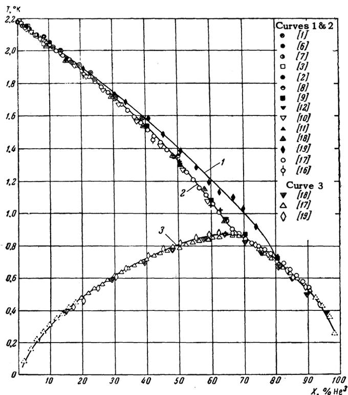
FIG. 4.  $T_\lambda(X)$  (curves 1 and 2) and  $T_p(X)$  (curve 3); data from the present paper are indicated by crosses (+).
