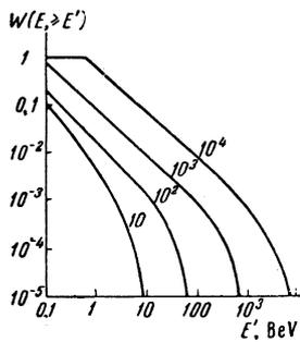
FIG. 4. Expected number of bursts with  $n = E'/\beta$  particles, produced by a muon with energy  $E$  under thick layers of iron. The numbers on the curves represent the muon energy in BeV.
