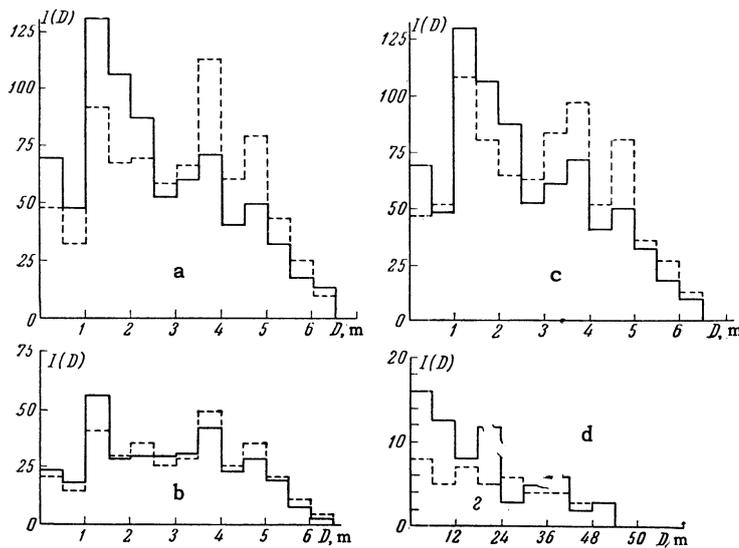
FIG. 2. Distribution of the distances  $D$  between the muon-registering counters: a—for  $R < 30\text{m}$ ; b—for  $R > 50\text{m}$ ; c—same as a, but theoretical distribution calculated with allowance for the angles of incidence of shower axes on the muon detector; d—part of the distribution a for  $D < 0.5\text{m}$ . Continuous curves—experiment, dashed—theory.
