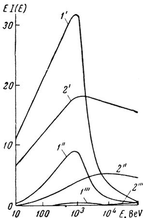
FIG. 3. Theoretically expected number of electron-photon showers produced by muons of energy  $E$ . 1—curves calculated for the muon spectrum given by (3), 2—the same for muon spectrum (4). Single prime denotes events of type V, Table I; double prime—events of type VII, Table I; triple prime—events of type F, Table II.
