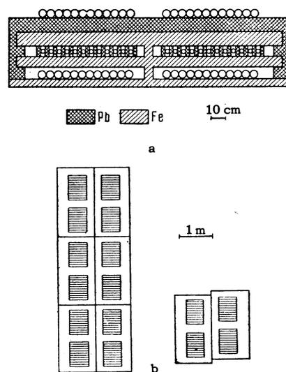
FIG. 1. Diagram of the setup: a—muon detector, b—arrangement of muon detectors in the underground chamber.
