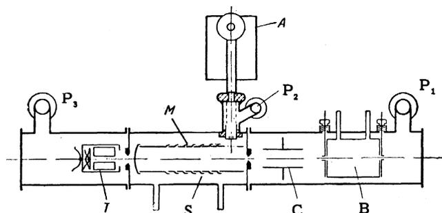
FIG. 1. Experimental setup: B is the chamber where an atomic beam is formed by charge exchange; C is the capacitor where charged particles are removed from the atomic beam; S is the scattering chamber; M is the measuring capacitor; T is the receiver of fast particles; A is the analyzer of slow ions;  $P_1$ ,  $P_2$ ,  $P_3$ , are pumps.
