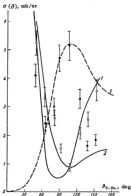
FIG. 3. Angular distribution of protons scattered from  $\text{Ca}^{40}$  excited to the levels  $3.352 \pm 0.010$  MeV ( $\circ$ , continuous curves) and  $3.733 \pm 0.014$  MeV ( $\bullet$ , dashed curve). Curve 1 – calculated with distorted waves ( $L = 0$ ); curve 2 – square of spherical Bessel function  $j_0^2(|k_i - k_f| R)$ ,  $R = 4.3 F$ ; curve 3 – square of spherical Bessel function  $j_2^2(|k_i - k_f| R)$ ,  $R = 6 F$ .
