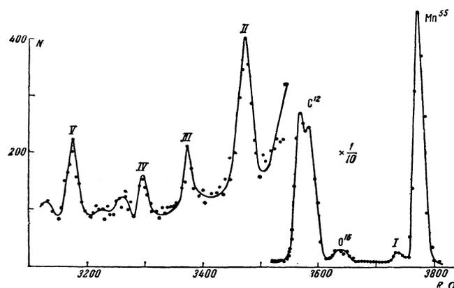
FIG. 1. Spectrum of protons scattered by a manganese target (with polystyrene backing) at  $\vartheta_{\text{lab}} = 79^\circ 50'$ . Abscissas represent resistances (in a resistance box) in the circuit of the analyzer-field meter. Ordinates are numbers of particles relative to a fixed number of counts of the beam-current integrator.
