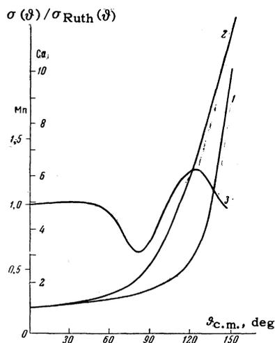
FIG. 2. Dependence of the ratio of the elastic scattering cross section to the Rutherford cross section on the scattering angle for  $\text{Ca}^{40}$  and  $\text{Mn}^{55}$ . Curves 1 and 2 – for  $\text{Ca}^{40}$  at  $E_p = 6.6$  MeV and 5.4 MeV, respectively; curve 3 – for  $\text{Mn}^{55}$  at  $E_p = 6.6$  MeV.
