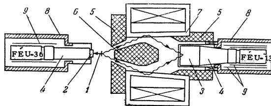
FIG. 1. Experimental layout. 1—Source; 2—stilbene crystal; 3—NaI (Tl) crystal; 4—light pipe; 5—lead collimator; 6—lead shield; 7—analyzing magnet; 8—Armco-iron shield; 9—perm-alloy shield.
