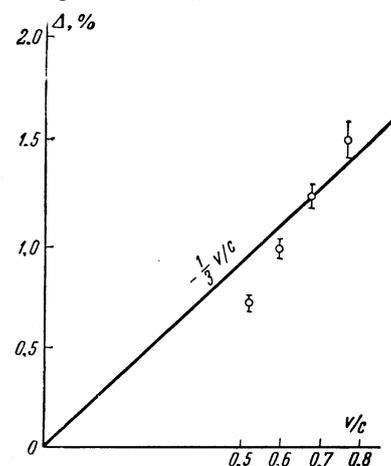
FIG. 4. Results of the measurements of the  $\text{Co}^{60}$  correlation coefficient.
