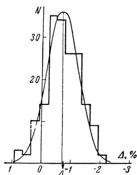
FIG. 3. Statistical distribution of the measurements for  $v/c = 0.52$  in  $\text{Co}^{60}$  during one hour. Point A denotes the value of  $\Delta$  determined from all the measurements. The ordinate axis gives the number of measurements.
