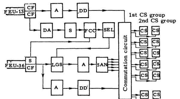
FIG. 2. Block diagram of apparatus: CF—cathode follower; S—signal shaping; DA—distributed amplifier; A—amplifier; DD—differential discriminator; FCC—fast coincidence circuit; SEL—selection circuit; LGS—linear gating selection circuit; CS—counting circuit; 5AN—five-channel amplitude analyzer;
