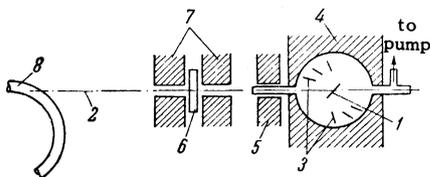
FIG. 1. Diagram of experimental setup; 1 – target, 2 – photon beam, 3 – nuclear emulsions, 4 – lead shield, 5 – poles of sweeping magnet, 6 – monitor, 7 – lead collimators, 8 – synchrotron.
