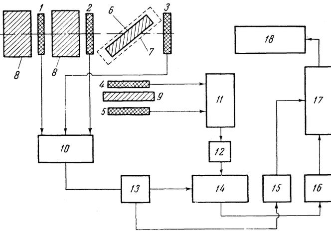
FIG. 1. Block diagram of apparatus. 1-5 - scintillation counters; 6 - target; 7 - magnetizing coil; 8 - copper absorbers; 9 - paraffin absorber; 10 - anticoincidence circuit; 11 - coincidence circuit; 12 - delay line; 13 - gate trigger; 14 - gate; 15, 16 - pulse shapers; 17 - converter; 18 - amplitude analyzer.
