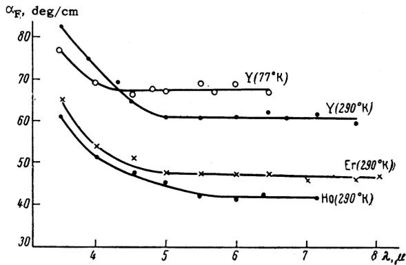
FIG. 1. Faraday effect in yttrium, erbium, and holmium garnets in infrared light at different temperatures;  $H_{ext} = 2400$  oe.
