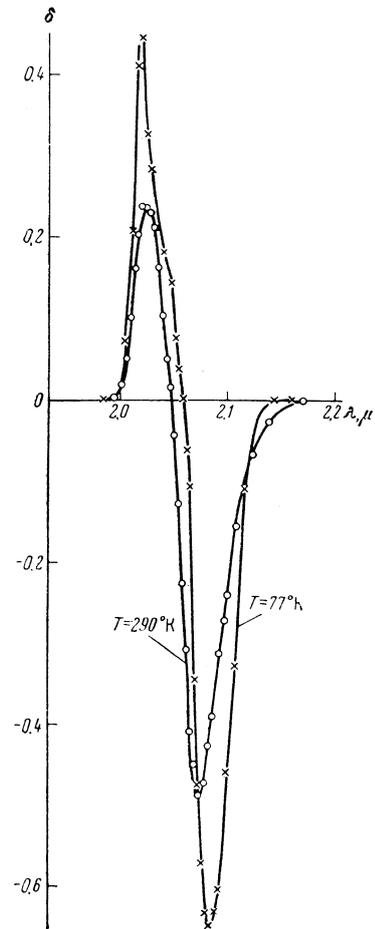
FIG. 3. Circular dichroism  $\delta = (\Delta_{\text{right}} - \Delta_{\text{left}})/\Delta_{H=0}$  of europium garnet in the absorption band region.
