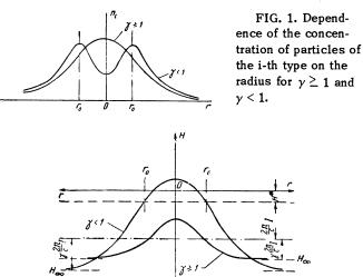
FIG. 2. Dependence of the magnetic field H on the radius for two cases  $\gamma \ge 1$  and  $\gamma < 1$ . As  $r \to \infty$ , the field approaches the constant value  $H_{\infty}$ .
