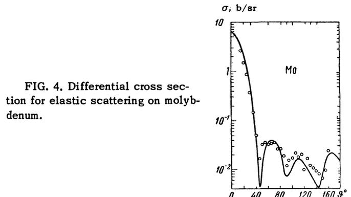
FIG. 4. Differential cross section for elastic scattering on molybdenum.
