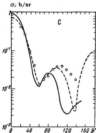
FIG. 1. Differential cross section for the elastic scattering of 14-Mev neutrons on carbon (in the laboratory frame of reference). Theoretical curves: the solid line in this and the following figures is taken from Bjorklund and Fernbach, the dashed line from Beister et al.<sup>[16]</sup>
