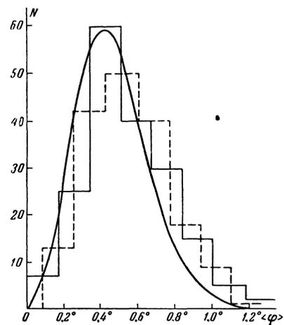
FIG. 3. Distribution of rms scattering angles on 200 tracks. The dashed and solid histograms were plotted for two groups of tracks selected at random. The theoretical curve was plotted for  $n = 3$  and  $\sigma_1 = 0.5^\circ$ .
