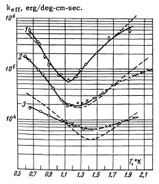
FIG. 5. Variation of the effective thermal conductivity of solutions of He<sup>3</sup> in He<sup>4</sup> with temperature and concentration: curves  $1 - \varepsilon = 1.39 \times 10^{-4}$ ; curves  $2 - \varepsilon = 1.32 \times 10^{-3}$ ; curves  $3 - \varepsilon = 1.36 \times 10^{-2}$ ; dashed curves are theoretical.
