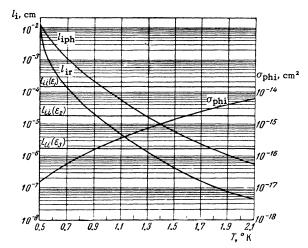
FIG. 6. Impurity mean free paths ( $\varepsilon_1 = 1.39 \times 10^{-4}$ ;  $\varepsilon_2 = 1.32 \times 10^{-3}$ ;  $\varepsilon_3 = 1.36 \times 10^{-2}$ ). Cross section for scattering of phonons by impurities as a function of temperature.
