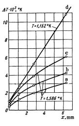
FIG. 4. Temperature distribution in reservoir for solutions of concentration  $\varepsilon = 1.32 \times 10^{-3}$  of He<sup>3</sup> in He<sup>4</sup>: a – for Q = 147.2; b – for Q = 212.1; c, d – for Q = 289.2 erg/cm<sup>2</sup> sec.
