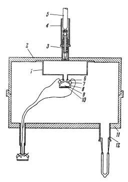
FIG. 1. Diagram of apparatus for thermal conductivity and diffusion measurements in  $He^3 - He^4$  solutions.
