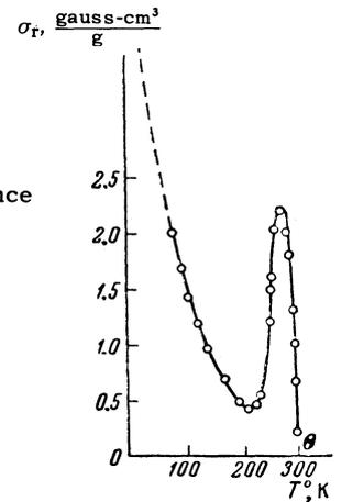
FIG. 8. Temperature dependence of the remanent magnetization of gadolinium.
