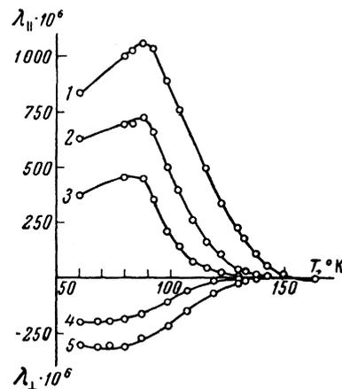
FIG. 4. Temperature dependence of the magnetostriction of dysprosium in constant magnetic field: curve 1 — longitudinal magnetostriction  $\lambda_{||}$  in a field  $H = 15,000$  oe; 2 —  $\lambda_{||}$  in a field  $H = 9,500$  oe; 3 —  $\lambda_{||}$  in a field  $H = 6,500$  oe; 4 — transverse magnetostriction  $\lambda_{\perp}$  in a field  $H = 15,000$  oe; 5 —  $\lambda_{\perp}$  in a field  $H = 9,500$  oe.
