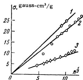
FIG. 11. The dependence of magnetization on  $H^{1/3}$  at the Curie temperature: curve 1 – Fe, 2 – Gd, 3 – Ni.
