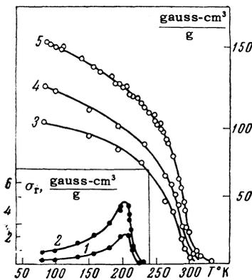
FIG. 6. Temperature dependence of the magnetization of gadolinium in different fields: curve 1 -  $H = 0.32 \text{ oe}$ , 2 -  $H = 0.64 \text{ oe}$ , 3 -  $H = 400 \text{ oe}$ , 4 -  $H = 1,000 \text{ oe}$ , 5 -  $H = 2,000 \text{ oe}$ .
