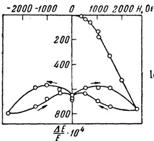
FIG. 2.  $\Delta E$ -effect hysteresis loop for dysprosium at 85°K.
