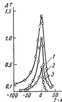
FIG. 12. Magnetocaloric effect near the Curie temperature: curve 1 – Fe, 2 – G, 3 – Ni.
